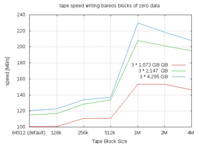
As can be seen, our tape device creates the maximum writespeed at a block size of 1M when writing bareos blocks with zero data.
